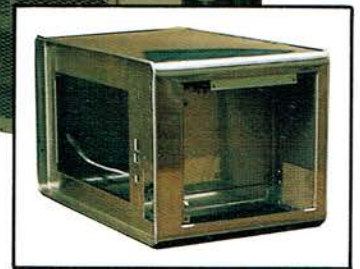
Finished microwave cavity
